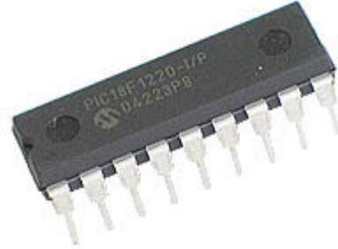
The chip is designed to be connected to a decoder (74HC154) and standard organ keyboard. It scans the keyboard and produces two oscillators and one trigger output - the chip can be connected to any Waveshaper/VCF/Envelope/VCA circuits to produce a monophonic analog synth.
