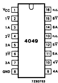
Fig.1 Pin configuration.
