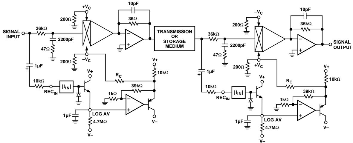
Figure 10. Companding Noise Rejection System
