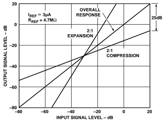
Figure 11. Companding Noise Reduction with 2:1 Compression/Expansion Ratio
