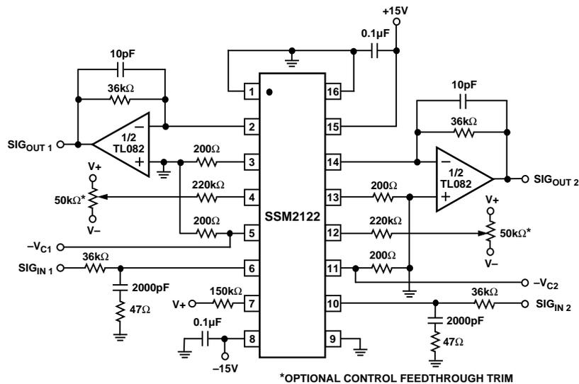
Figure 16. SSM2122 Basic Connection (Control Ports at 0 V)
