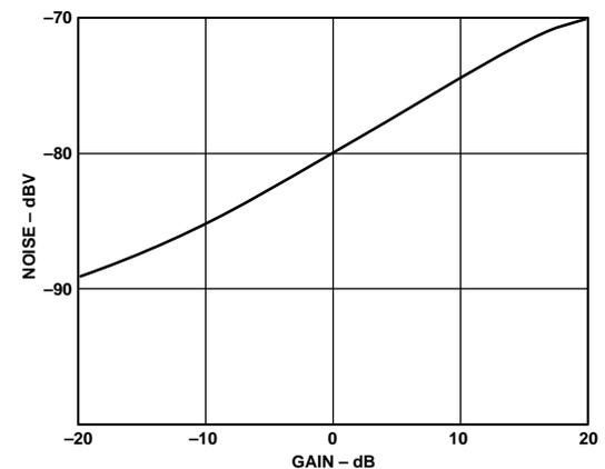
b. VCA Noise vs. Gain (20 kHz Bandwidth)
