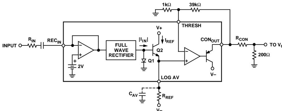
Figure 3. Level Detector
