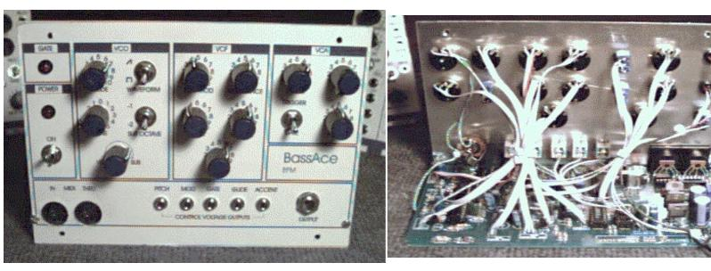
The BassAce is a small midi-synth based loosely on the TB303. It can be built many different ways. Depending on how it's configured it can be anything from a simple 303 type box to a full scale mono-synth. The 1/2 FracRac((TM) PAiA) shown here is in the maximum configuration without adding more pc boards. I have included a version of this layout for use with a Hammond case at the end of tis document. Add a VCO4 board, a Dual EG and a small mixer and you've got a full 2-VCO synth.
