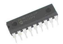
The chip is designed to be connected to a decoder (74HC154) and standard organ keyboard. It scans the keyboard and produces two oscillators and one trigger output - the chip can be connected to any Waveshaper/VCF/Envelope/VCA circuits to produce a monophonic analog synth.
