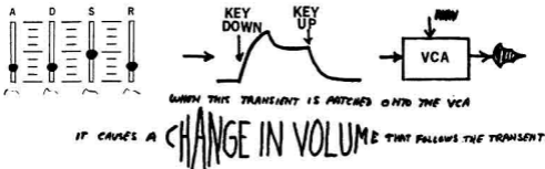
FIG. 18- The patching of the ADSR transient onto the VCA causes the loudness of the synthesizer to vary according to the transient shape.
